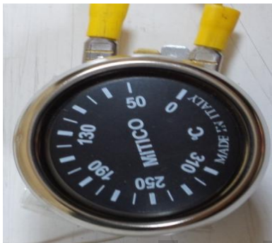
Fig (4): The electric thermostat attached to the electric circuit of the heating coil.
