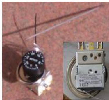
Fig (4): The electric thermostat attached to the electric circuit of the heating coil.
